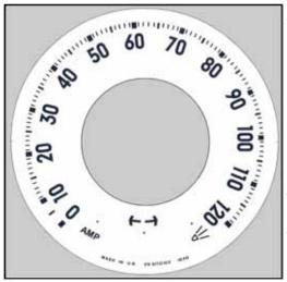
Look at the speedo overlay. You will find two small marks on the outer edge. One at 23 MPH and another at 101 MPH. On a 200 km/h speedo, the marks are at 36 and 166 km/h. Locate these positions on your metal speedo face and use a sharp tool to scribe very small marks in the same two posi-
