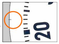
tions at the outer edge of the face plate. The face is brass under the paint. The marks should be made visible so you can see them when positioning the overlay.
