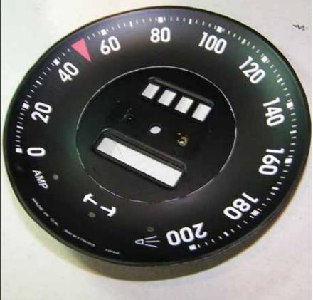
After you are satisfied that the overlay is in place, not use your hair drier again to heat the entire face. The overlay can safely heated to 175 degrees Fahrenheite (80 Deg C). Heating the vinyl in this way will help to set the shape of the overlay so that it does not try to resume a flat shape.
