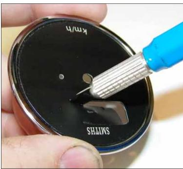
Your next step will be to cover the speedo center disc. The three round center holes will already be cut out for you. Use those holes to line it up. And be careful to make the edges even around the inside of the chromo
