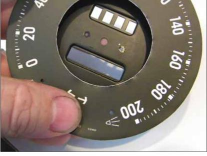
You will notice that the small holes in the overlay for the three warning lamps are not yet fully cut out. This will be finished by you later using a sharp hobby knife. The small wire you see at the ZERO position is a limit stop for the speedo needle. It needs to be pulled from the hole.
