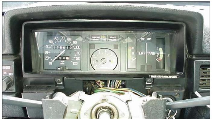
You may now reach up to the back of the speedo and find a plastic retainer on the cable end which attaches to the speedo. This retainer needs to be twisted approximately 1/4 turn counter-clockwise to release the cable from the speedo. The cable may then be pulled free from the speedo.
