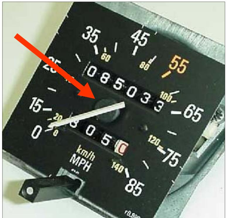
The needle can be moved back and forth, while gently pulling, until it comes off the shaft.
