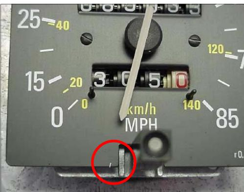
Make a note of where the needle rests. There may be a **small calibration mark** at the bottom of the face and the needle should point to it. This will be **very important for reassembly** as this is the position you will place the needle back on before lifting it back over the pin to the zero position.
