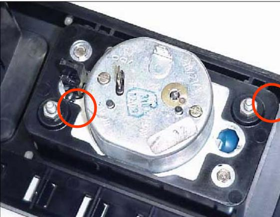
To disassemble the clock, remove the screws on the back. On some clocks, such as the one shown, there are two hex screws and two hex studs (5.5 MM or 7/32 inch). On others, there will be just two slotted screws. Next, gently pry off the two needles. They will come off easily. A small screwdriver works fine for these.
