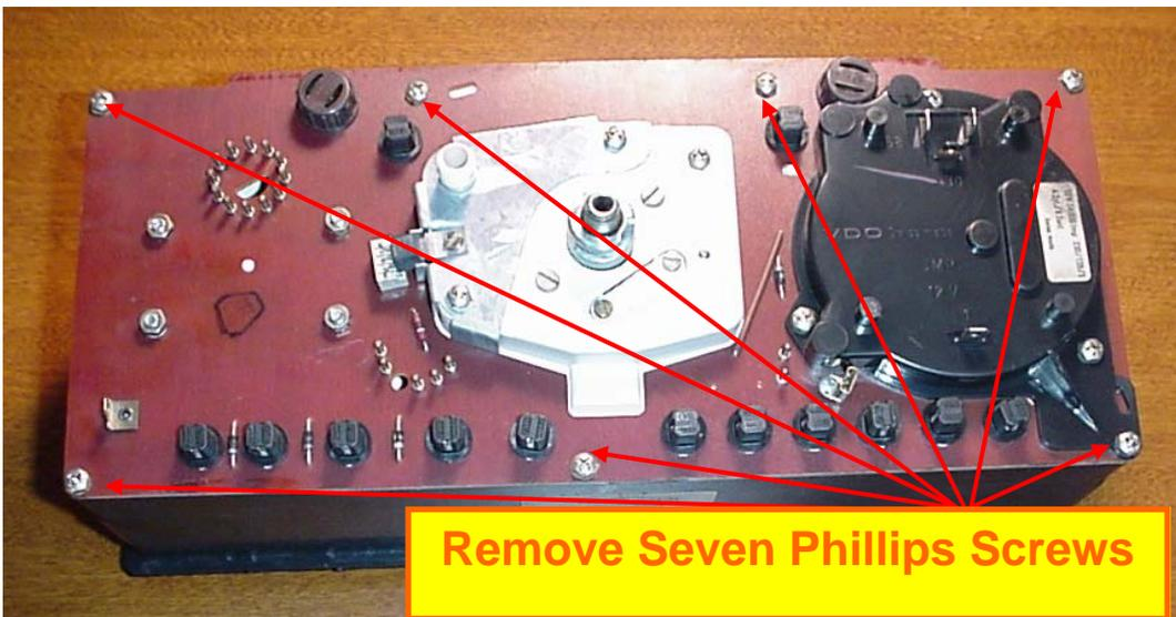
Turn the gauge pod over and locate the seven Phillips head screws on the outer edge. Removing these screws will allow you to lift out the **gauge/circuit board assembly** from the pod box.
