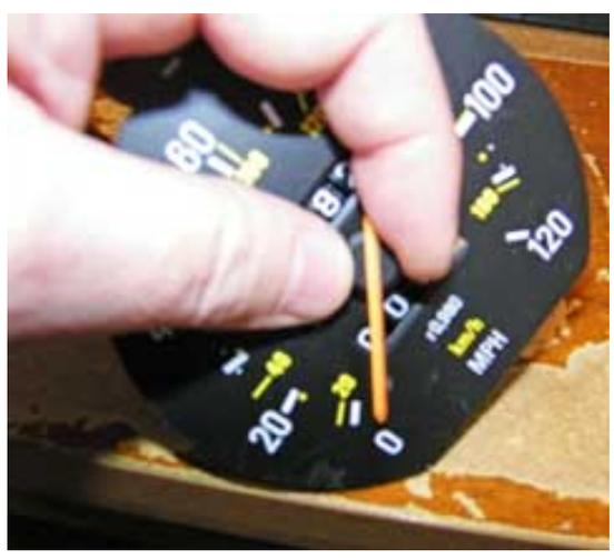
Now, grip the center plastic hub of the speedo needle and turn it counter-clockwise (toward the "MPH"). Be careful not to put pressure on the orange needle pointer. It's plastic and will snap off if you do.
