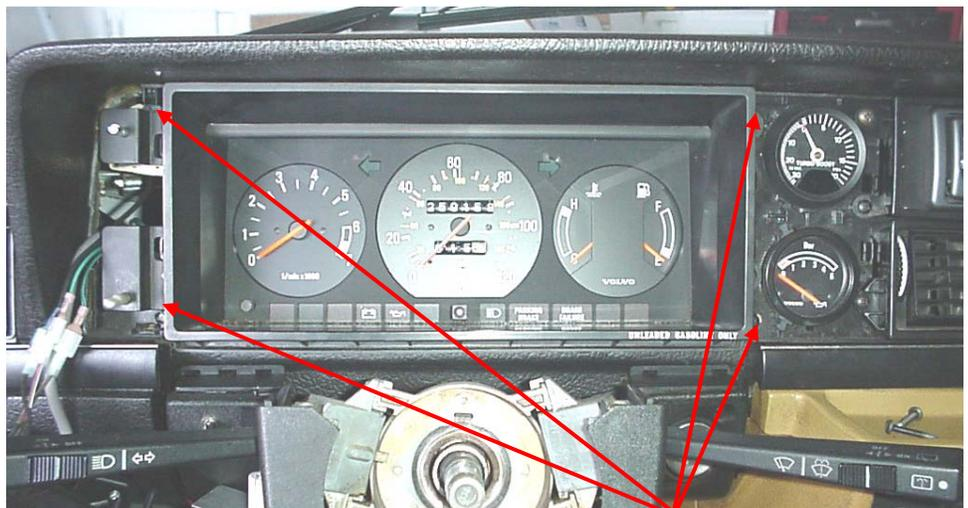
signal and wiper controls. There are two Phillips head screws on top (T-25 Torx screws for later cars). Now the gauge pod may be gently pulled toward you. It will be tight at first, so some pushing from behind will help. Pull it out enough so you can see the wire plug connections on the back. **Take note of each connection so you will remember exactly where they go.** Writing them down is best. Now disconnect the wire connections.
