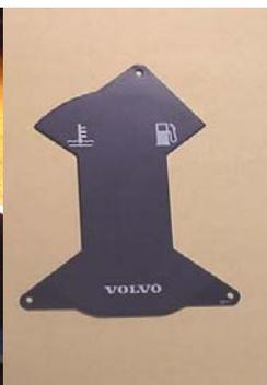
Please read and consider the section above about using an **optional adhesion promoter** on the edges. Test fit the new overlay first, then peel and apply it.
