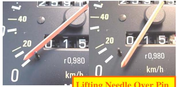
Your speedometer needle is tightly pressed onto a very small shaft in the speedometer. **It is on tight. DO NOT ATTEMPT TO PULL IT OFF WITH YOUR FINGERS, PLIERS, TEETH, ETC.** If you do, you will **BREAK** the needle...
