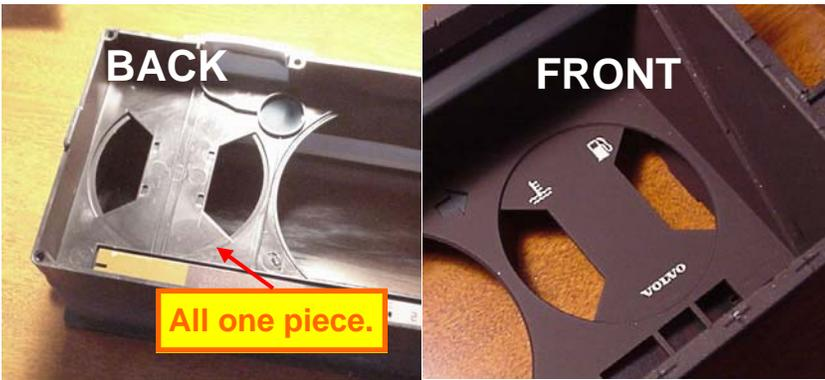
You will notice that this later gauge gauge box has **no removable metal plate** between the Temp and Fuel gauges. This plate is plastic and one piece with the box. **I have designed and cut the overlay to fit correctly. It will be mounted from the front instead.**
