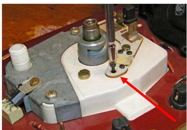
Locate and remove a small slotted screw on the back, near the bottom of the speedo. Insert a small slotted screwdriver down into the hole.
