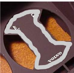
**Always test fit the overlay first, then peel the liner and apply it.**
