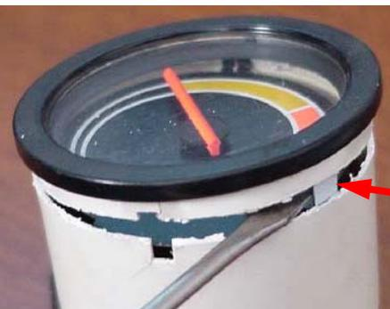
**NOTE:** If you are cutting an OEM VOLVO 240 Turbo Boost Gauge, you will need to cut a little closer to the ring. Make your cut on this gauge about 3/16" from the ring.
