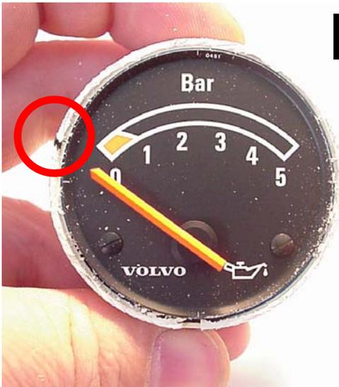
**6** Notice that a mark has been placed with a felt pen on the edge of the housing? This mark should be to record the position of the needle at rest before removing it. It will be used later for lining up the needle when you reassemble it.
