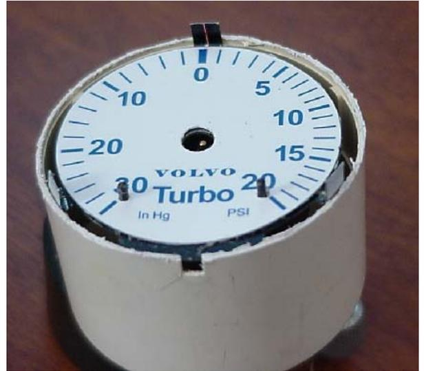
For other gauges, replace the face on the gauge and gently tighten the screws. These screws do not need to be really tight, so just make them snug.
