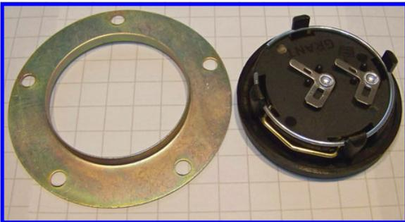
An alternate method can be used if the brass bar will not be resting against metal, or if the metal it touches doesn't complete your circuit. With this method, you will simply find a way to secure a wire to the common or grounded portion of the column. The other end of the wire is then connected to the (B) connector.
