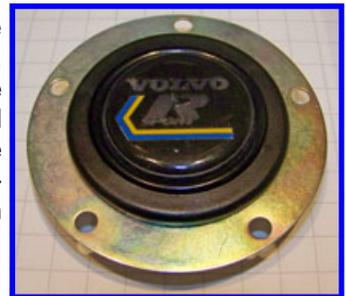
Connecting a wire to the common portion of a column can be as simple as crimping on a ring terminal and bolting the terminal to an outer hole in the hub when the steering wheel is bolted down. A MOMO steering wheel typically has 6 such bolts. A Grant wheel usually has 5 (the metal ring shown is for a Grant wheel).
