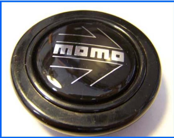
This horn button is very simple. It's just a switch. Open or closed. Open is off. Closed it on. When closed, it completes the electrical contact (or circuit) for a horn. There are a couple ways to hook things up to the back of this button. I'll cover both here.
