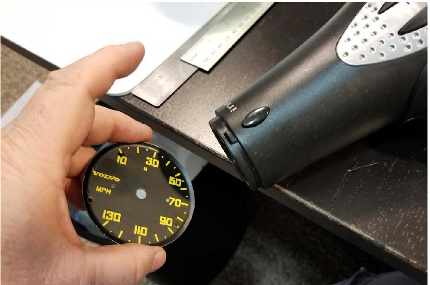
I use the below burnishing tools when installing face labels. Something like this works much better than using your fingernails. Any small, smooth tool could be used. Very light pressure is needed, but be careful not to rub hard as you could scuff the new label.
