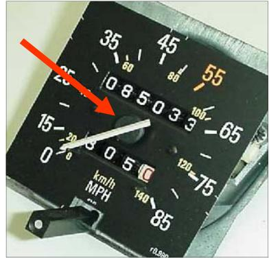
Using a very small flat blade screwdriver, remove the **two small screws** holding the face-plate to the speedometer. These screws are a soft brass, so try not to gouge the screws (or the face). Keep these screws **separate** from the screws for the tachometer as they are different lengths. Remove the speedometer faceplate and set it aside.
