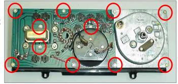
Lift out the **tachometer** first. It's held snug by two pins for the electrical current connection. Pull and it will come out.
