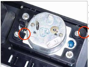
To disassemble the clock, remove the screws on the back. On some clocks, such as the one shown, there are two hex screws and two hex studs (5.5 MM or 7/32 inch). On others, there will be just two slotted screws. Next, gently pry
