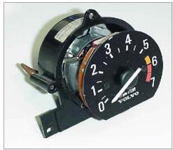
Gently grasp the needle with your fingers at the **center**. Twist the needle counter-clockwise. It will give a slight amount of resistance, so **don't put pressure on the plastic needle pointer as it can break off**. While twisting the needle in a counter-clockwise direction, pull toward you. The needle will eventually pull off the small shaft. Re-installation is as simple as pushing the needle back on the shaft and pushing with your thumb.
