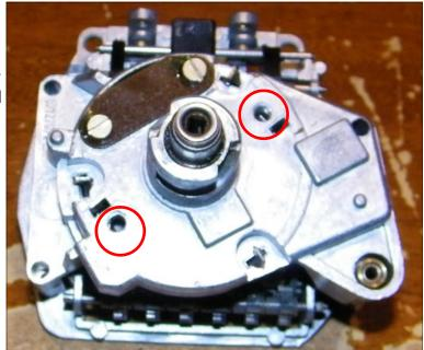
Now you should grasp the center round section of the needle. To remove the needle, you will turn it in a direction away from the stop pin at zero. Either direction is fine, just don't break the pointer arm on the pin. Some force will be necessary to release the grip on the shaft. Be very careful NOT to put pressure on the plastic needle pointer arm or it will break off.
