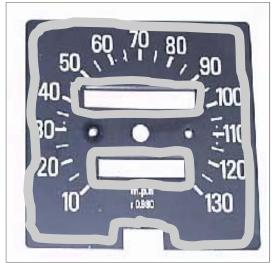
Application should be done with a swab along the edges, like shown here. It dries clear and provides a better surface for the labels. Allow it to dry, then apply the labels.
