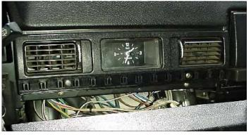
Remove them. Now you may pull the whole clock/vent assembly toward you. After pulling it out a few inches, look at the wire connections on the back of the clock. There are **two light bulbs** and **two connectors** for the clock. Write down where these connectors go. The light bulbs may be twisted 1/4 turn counter-clockwise and pulled out. The two clock connections simply pull off.
