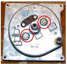
Turn the speedo over and remove the two slotted screws shown and separate the back plate from the speedo.
