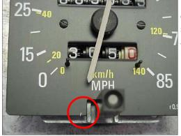
Make a note of where the needle rests. There may be a **small calibration mark** at the bottom of the face and the needle should point to it. This will be **very important for reassembly** as this is the position you will place the needle back on before lifting it back over the pin to the zero position.
