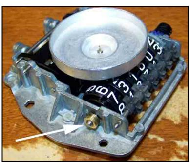
See this brass collar? It's pressed onto the shaft (opposite end from the outside gears). This shaft goes through the odometer number wheels and through the two outside gears on the other side. When you try to spin the outside gears (while holding the wide black inside gear steady), have a look at this collar to see if the shaft/collar is spinning along with them.
