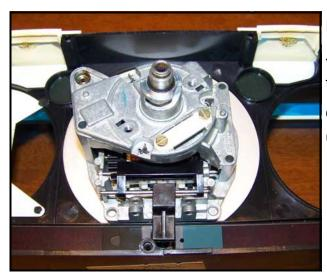
Lift out the circuit board.
