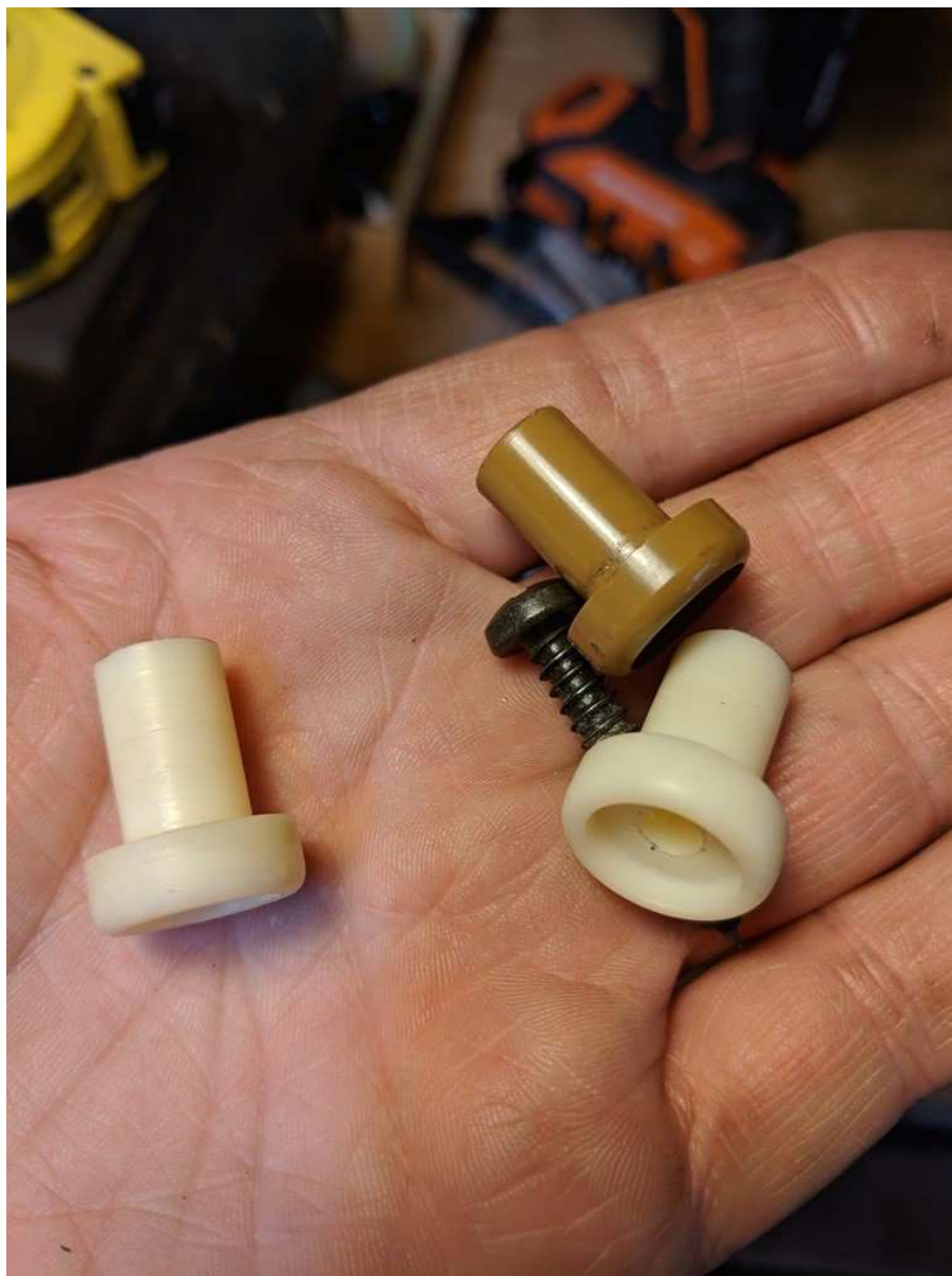
I turned out a couple of replacement map pocked bosses, painted them, and the map pocket (it was brown before) black and began reassembly on car.
