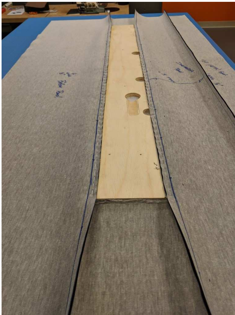
Here you can see the wrap on the intermediate raised relief panel. This panel, its batting, and the entire stitch vinyl become a sub assembly that gets attached to the door card after stapling.
