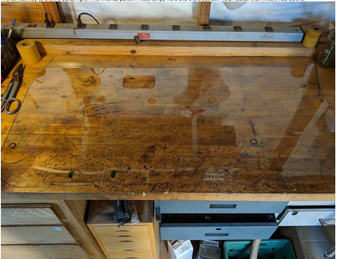
I had tried to copy the old panel which was a complete disaster, it was so warped and rotten(failure#1). I then tried clear shower curtain vinyl to cut the holes directly from the door but the vinyl was too soft to stay flat and accurate (failure#2). I then ordered a sheet of 0.040 poly-carbonate which was stiff enough to hold its shape, mount components to, and easy to score lines and cut shapes from. I stuck the PC sheet to the door to transfer holes and features using double sided foam tape, the same 3M stuff you use to put on weatherstripping and trim. Tip: run a rag over the tape once
