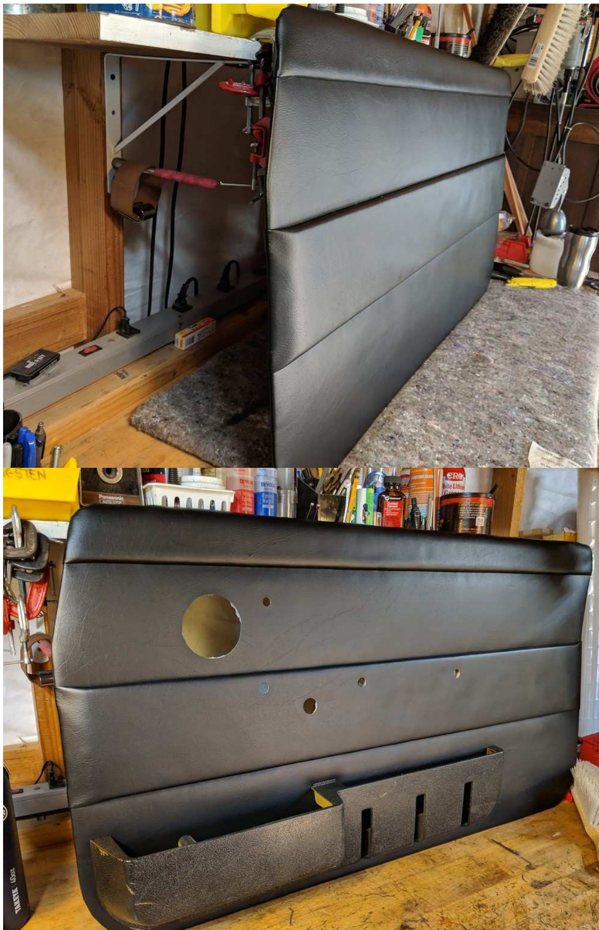
I cut the holes with a hole punch set and a set of dividers with an xacto blade taped to one side. I left the interior handle recess to be cut once in to make sure I didnt cut more than I needed to. The handle bezel actually acted like a near perfect cut template.
