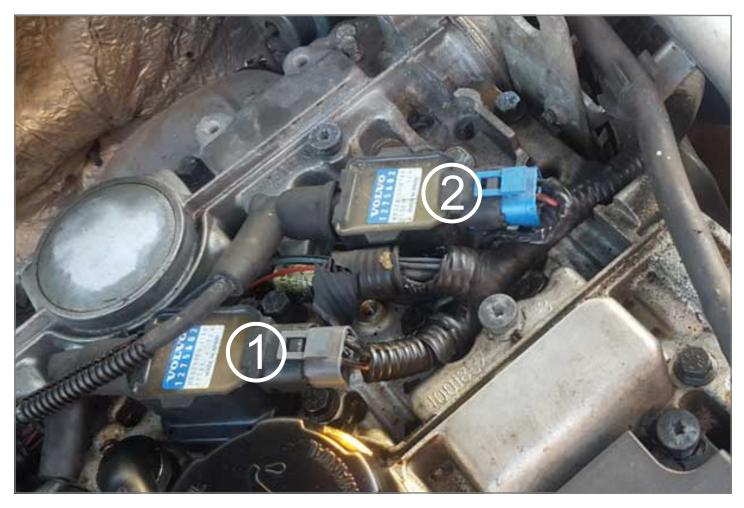
decide to use it, it must be slide over the wires before splicing. I recommend using the heat shrink tubing on two wires for one coil, and then on two wires for the other coil. If you cannot get enough free length of the old wire to fit heat shrink tubing, then you may use electrical tape to seal the splices after.
