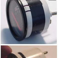
With a hack saw, slowly cut through the gauge housing, rotating the housing a little as you go. Be careful... don't allow the blade to go too deep; just allow it to break through the surface of the housing. Take your time.
