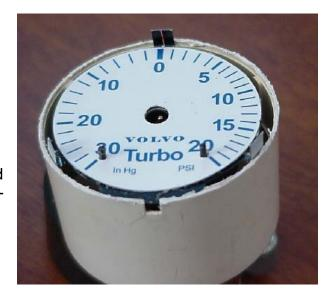
For other gauges, replace the face on the gauge and gently tighten the screws. These screws do not need to be really tight, so just make them snug.
