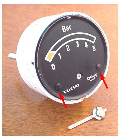
To remove these little screws, use a <u>proper</u> <u>fitting</u> small screwdriver to remove them.
