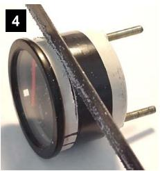
After cutting is complete, separate the two halves.
