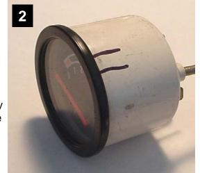
Measure about 1/4 inch away from the metal ring and place some tape around the gauge for a cutting guide. A simple marker line works OK too.
