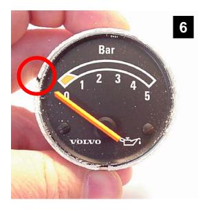
Notice that a mark has been placed with a felt pen on the edge of the housing? This mark should be to record the position of the needle at rest before removing it. It will be used later for lining up the needle when you reassemble it.
