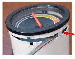
**NOTE:** If you are cutting an <u>OEM VOLVO 240 Turbo Boost</u> <u>Gauge</u>, you will need to cut a little closer to the ring. Make your cut on this gauge about 3/16" from the ring.
