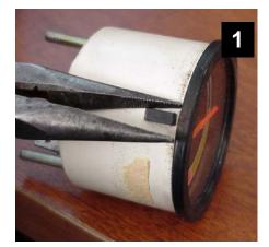
If your gauge has this plastic guide piece on the bottom, remove it. Simply pull it off with pliers.
