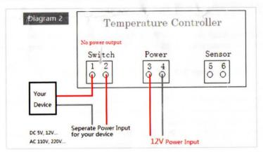
The following diagram is a typical wrong circuit wiring:
