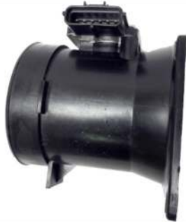
Example MAF #3: 6-Pin Ford, Internal IAT Sensor (unknown size)
