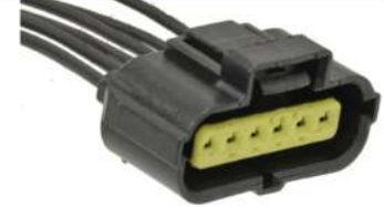
Example MAF #3: 6-Pin Ford, Internal IAT Sensor (unknown size)
