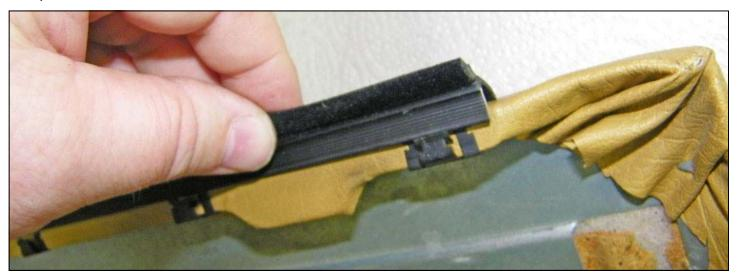
NOTE: The width of the new scraper may be a little wider than your old one and it may protrude past the door lock plunger collar as shown in the below photo. If this happens, you may tuck it under the door lock insert using a small screwdriver.
