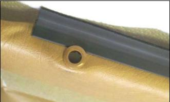
Here's a tip that might be useful for a door panel that doesn't seem to hold the scraper as snuggly as it should to the glass. In this situation, the scraper may end up with a gap where the felt should be actually be touching the glass. If this happens, those two metal tabs shown below may have become bent away from the glass. You can then try (slightly) bending the two metal tabs a bit toward the glass.
