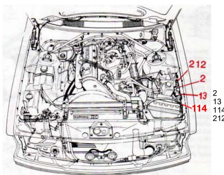
Power junction box (12v from battery) Headlight relay (stepped high/low beam) Cooling fan relay (AC) Main relay, LH fuel injection
